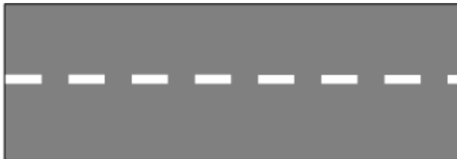
Figure 19 - Runway Centre-line Markings
