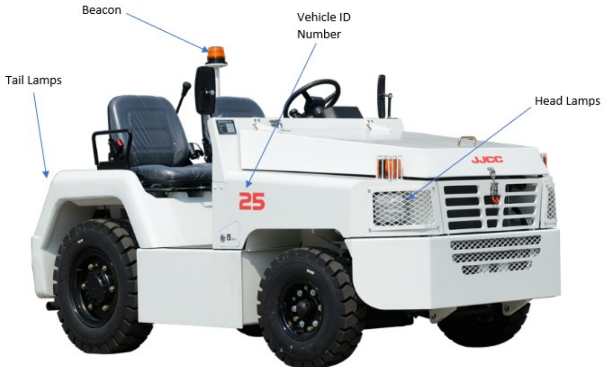
Figure 6 - Vehicle without a Cab Required Safety Markings and Lighting
