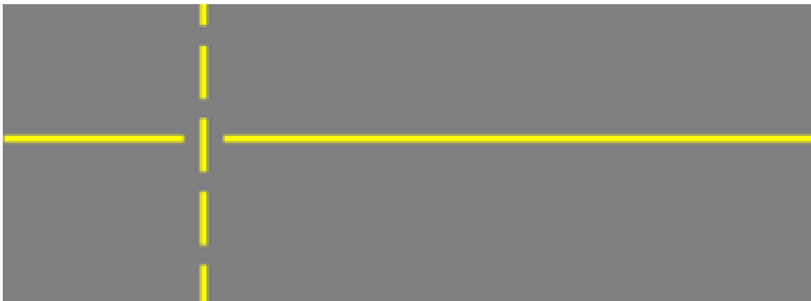
Figure 16 - Taxiway Intersection Marking
